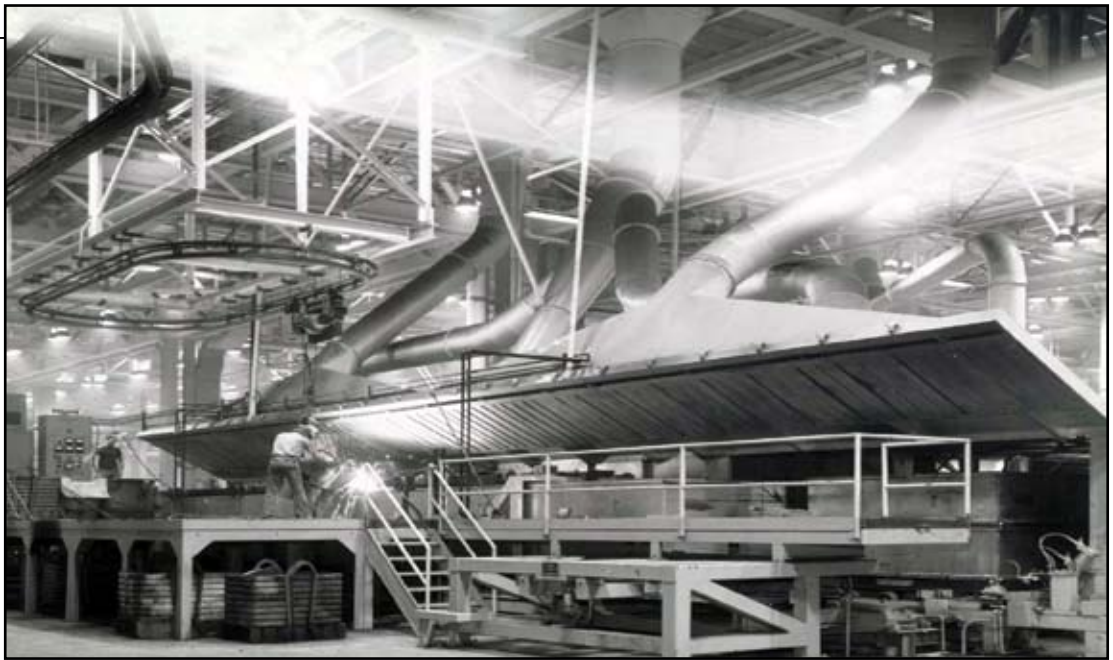
FIGURE 2. Hoods that cannot be designed with total enclosure should be located as close to the source as possible. A side draft hood located twice the distance from the source can require as much as four times the exhaust volumetric flowrate
