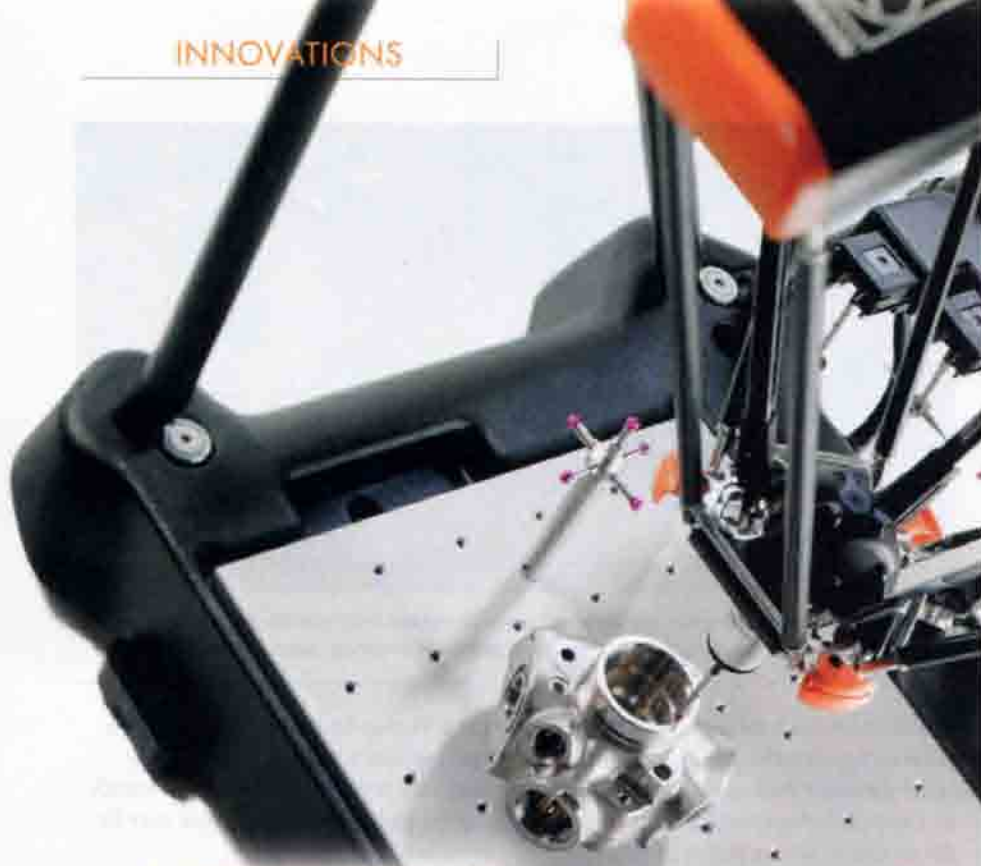
◀ The Equator uses a parallel kinematic structure for high-speed scanning and repeatability. Source: Renishaw
