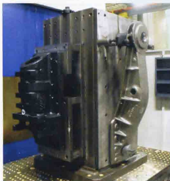
A wide variety of thread mills, boring bars and some customized tooling are used to machine the drawbars and other railway components on a tombstone fixture.
