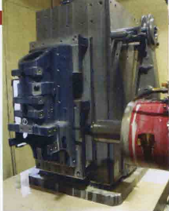
The 31.5 in live-spindle reach eliminated a second machine and setup, allowing engineers to add the yoke of the drawbar assembly on the pallet, which freed up another machine in the process.
