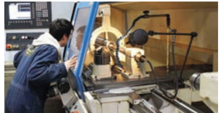
Cougar Tool bores up to 30 inches depth using this setup on a MAG VDF 560 DUS lathe, though usually works to a depth of 24 inches. This hydraulic housing is bored from both ends to complete the part, then sent out for chroming and honing of the ID.
