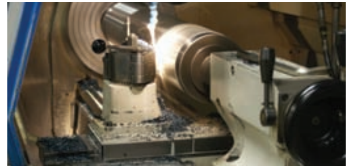
MAG VDF DUS lathe machines the OD on a DJ10 piston sub. After OD machining, operator will setup steady rest and bore the ID. Part would then be sent out for hard chroming and honing of the ID, where a polypack seal runs.
