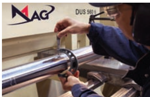
Operator measures OD on a latch mandrel after turning on a MAG VDF 560 DUS.
