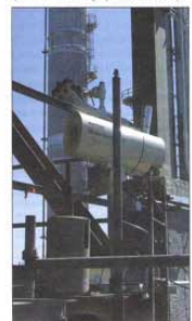
The largest radiometric imaging system for safety monitoring of a petrochemical processing vessel uses 14 Mikron infrared cameras and MikroSpec R/T software. It has been online for more than a year monitoring this Chevron-Texaco-designed gas separation system in Texas.
